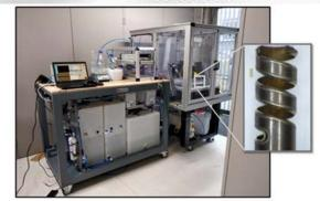
DEFINE-AM platform and sample jECM machined stainless tube developed during DTIF
