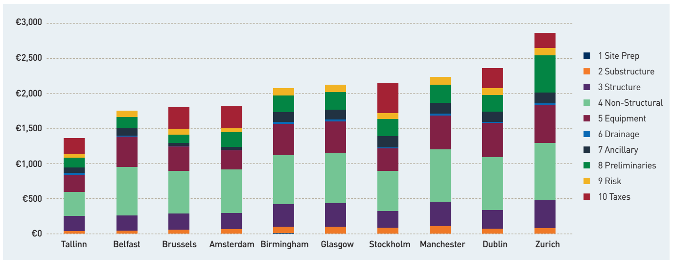
Figure 2: Cost per m 2 , by ICMS3 Group and city. Source: Analysis of survey results.
