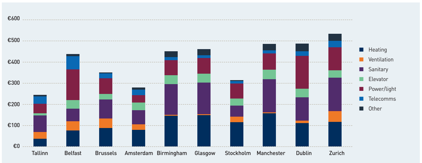
Figure 4: Services and equipment costs per m 2 , by cost type and city. Source: Analysis of survey results.
